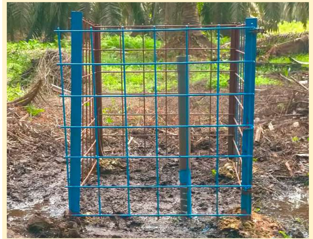
Subsidence Pole is installed to measure the subsidence rate of the peat
