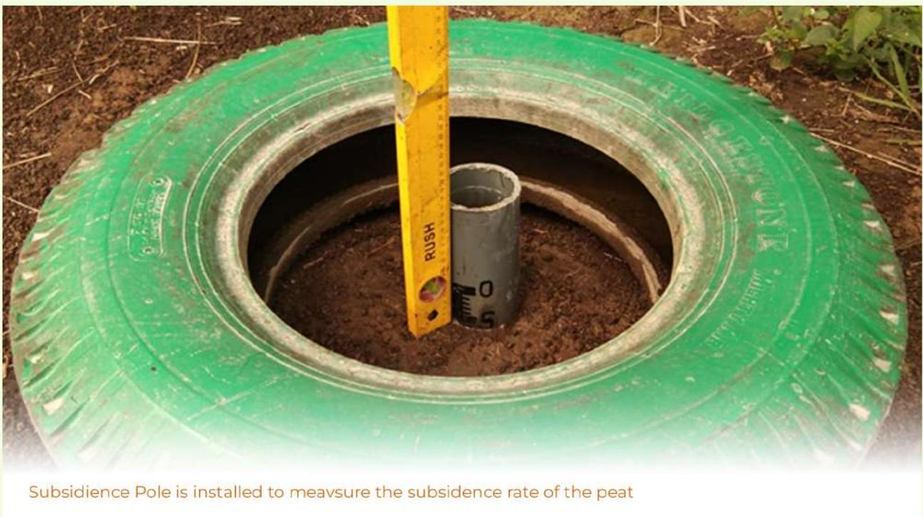
Subsidence Pole is installed to measure the subsidence rate of the peat
