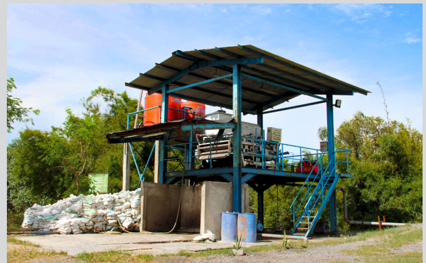
Belt presses are installed in some of our mills to help reduce effluent's COD load
