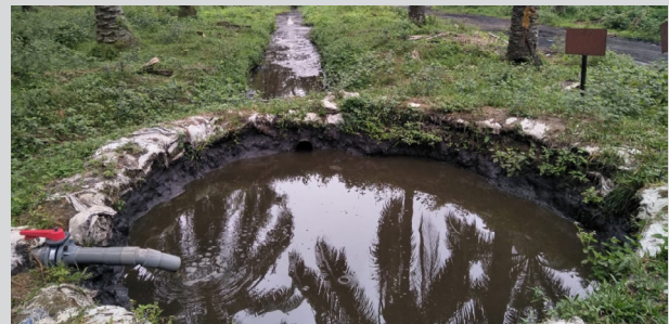
Our land application systems recycle the nutrients present in POME back into the plantation
